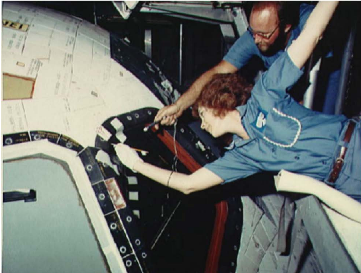
Figure 17O-4 Repairing TPS on Columbia
